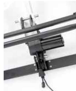
Motor fixation with 2 axis
